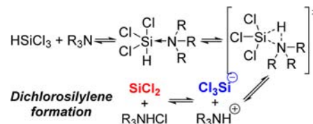
Scheme 4. Generation of SiCl 3 − and SiCl 2 from HSiCl 3 in the Presence of Tertiary Amines
